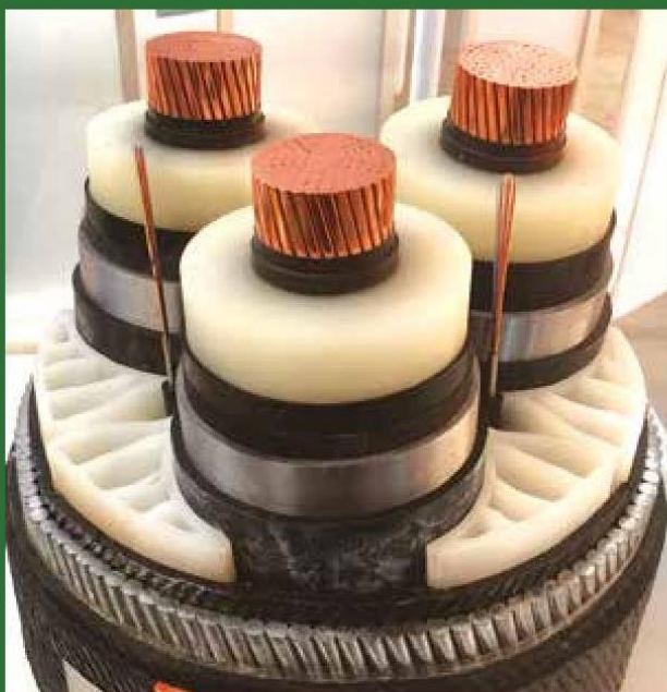
Combination of three single core land cable to a 3 x 1200 mm 2 AC submarine XLPE cable 220 kV for wind park connection.
