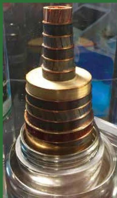
Superconducting cable for 138 kV and 2400 A.
