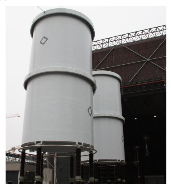
Coil Innovation, the leader in the air-core dry-type technology has successfully type tested its first 420kV air-core dry-type shunt reactor, which will be delivered to a German Transmission System Operator.
